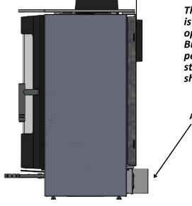
The stove requires a permanent air vent to the room. This is to provide adequate air supply in order for the stove to operate safely and efficiently. In accordance with current Building Regulations the installer may have fitted a permanent air supply vent into the room in which the stove is installed to provide combustion air. This air vent should not under any circumstances be shut off or sealed.
