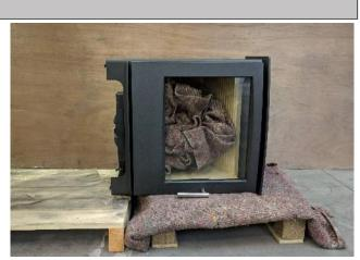
Tilt the stove onto it's side to allow easy and safe access to the feet. Unscrew the levelling bolts at the foot of the stove leg.
