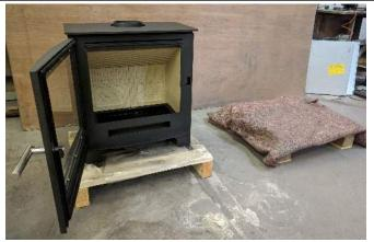
Remove the internal components of the stove and fill the chamber with material to prevent the bricks from falling. Additionally, prepare a soft elevated surface.
