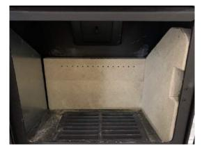
It is now possible to remove the top baffle brick by lifting up the left side and sliding it to the left then dropping it down. The right hand side brick can be removed by gently pulling it down from the top.
